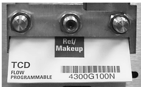
Figure 4. Gas line connections
